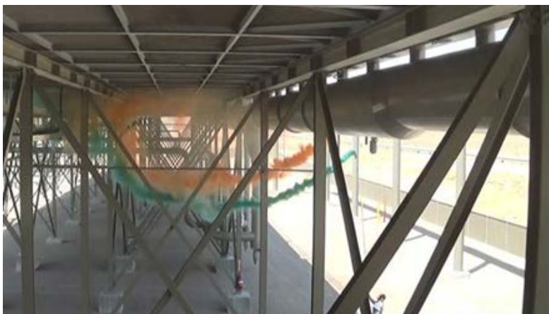
Figure 10 - Air inlet streamlines in cross wind WGV
