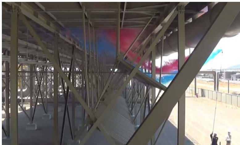
Figure 10 - Air inlet streamlines in cross wind WGV
