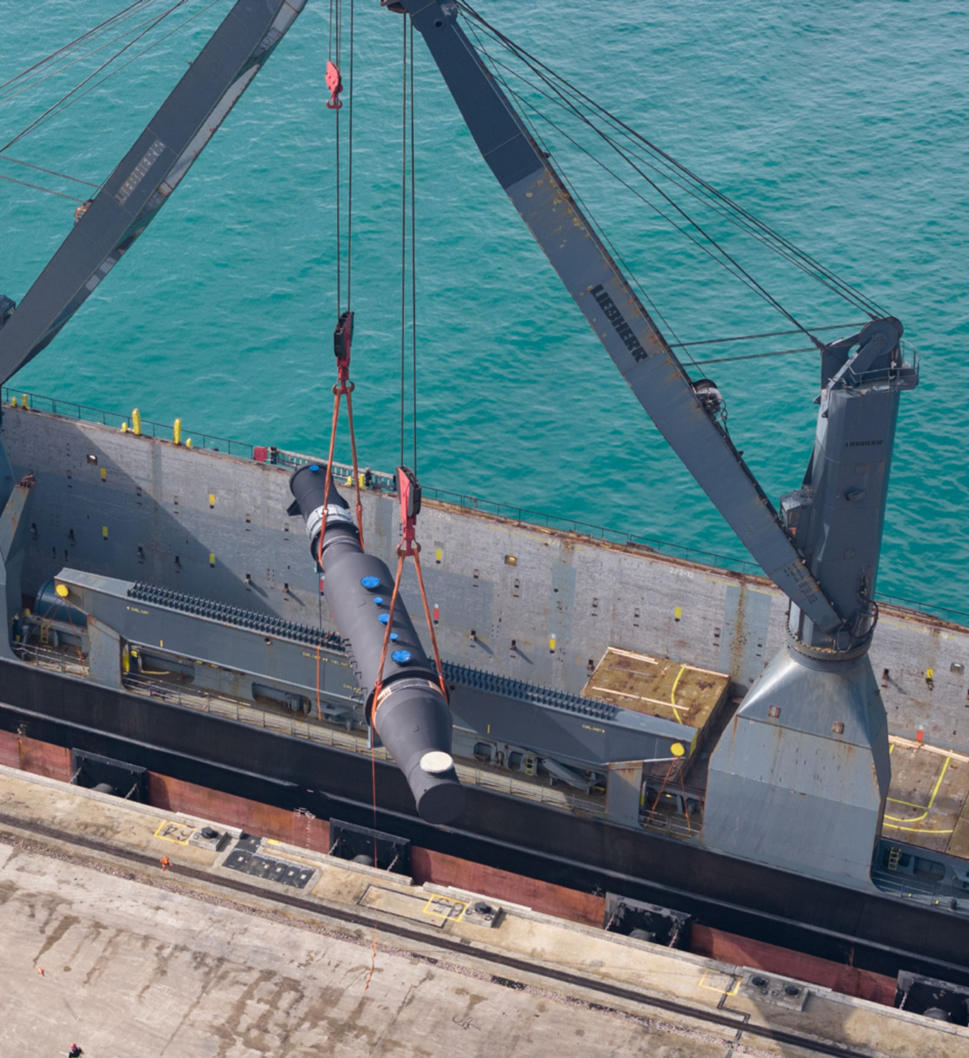
Te mihi Heat exchanger loading
